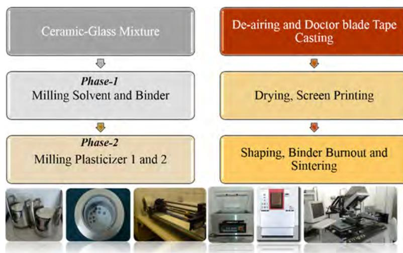
Figure 1. Tape casting processing flow chart.
